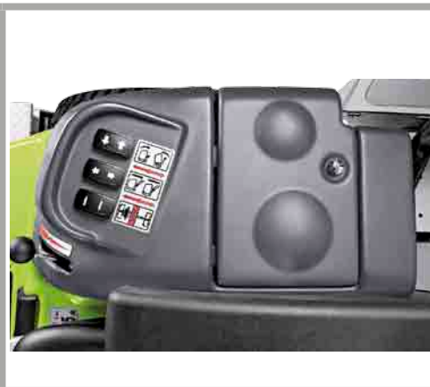
Controls via electric buttons
