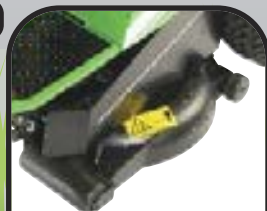
Cast aluminium deck
