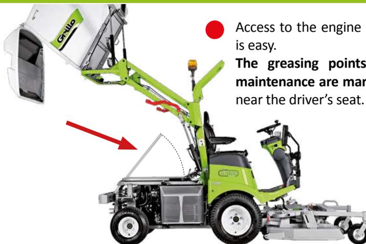
● Access to the engine compartment is easy. **The greasing points for routine maintenance are marked in a label near the driver's seat.**
