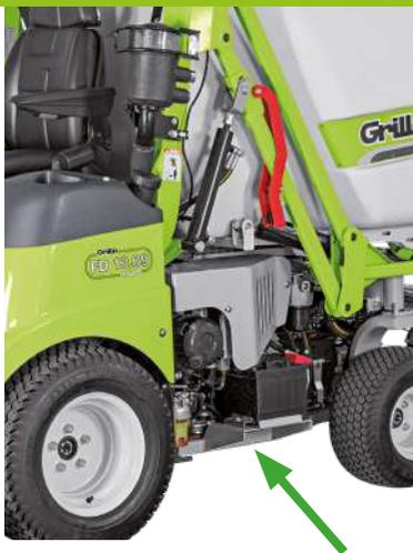
● **Access to the pre-filter, the engine air filter, the diesel filter and decanter and the hydraulic oil filter is easy.** Even the battery is easily accessed, as well as the belt tensioner and the hydraulic PTO clutch.
