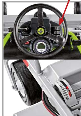
Hydraulic-assisted and continuous cutting adjustment
