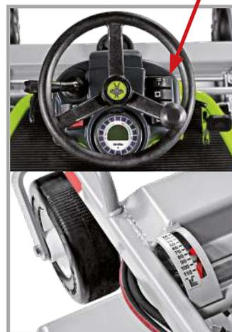
Hydraulic-assisted and continuous cutting adjustment
