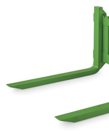
"Click & go" front loader mounting comes as standard and could not be quicker, safer or more convenient, thanks to the patented self-correcting floating system of the built-in automatic mast latch.
