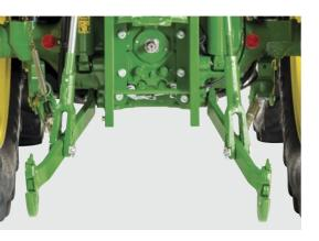
Hook up whatever you need for the job. Built to handle even the heaviest of implements, the super robust rear hitch of the 5M has a maximum lift capacity of up to 4,440 kg (maximum lift capacity at hooks).
