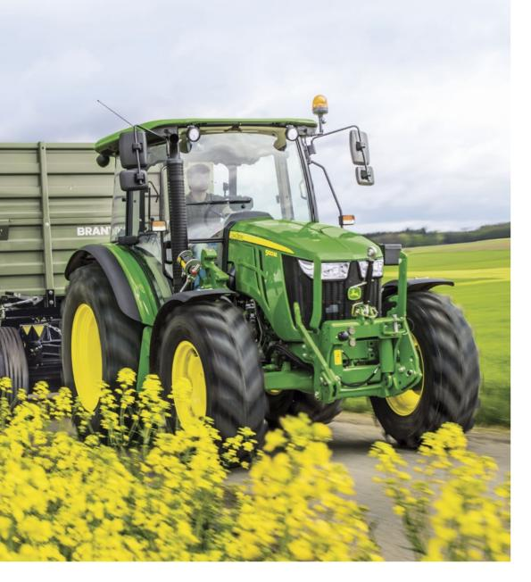
No additives required. By combining Cooled Exhaust Gas Recirculation (EGR) technology with an intercooler and Diesel Particle Filter (DPF), Stage IIIB emissions standards are met without the need for any additives.
