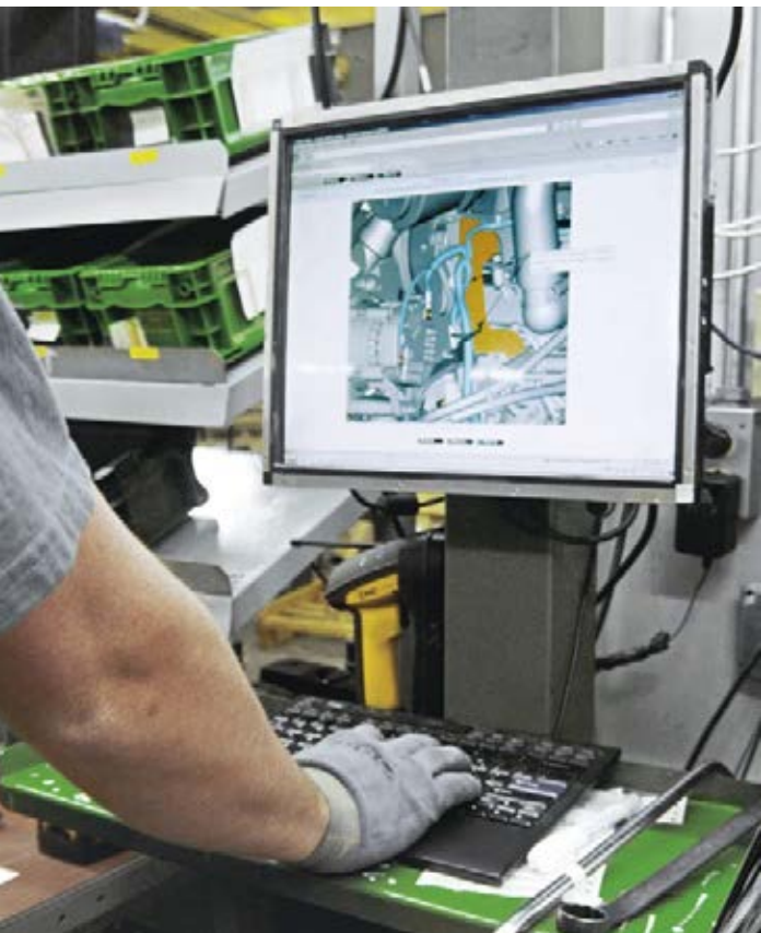
Every station has a computer display that shows operators what to do next in pictures and animations.
