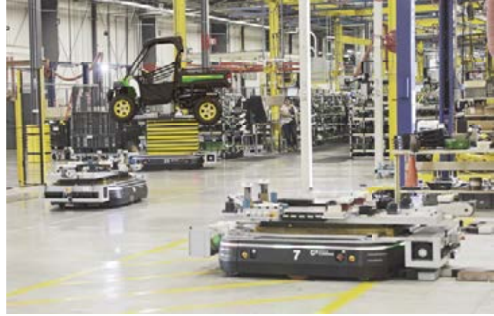
A mobile robot called OTTO recharges at a docking station. OTTOs ferry components around the assembly line constantly to keep production smooth.
