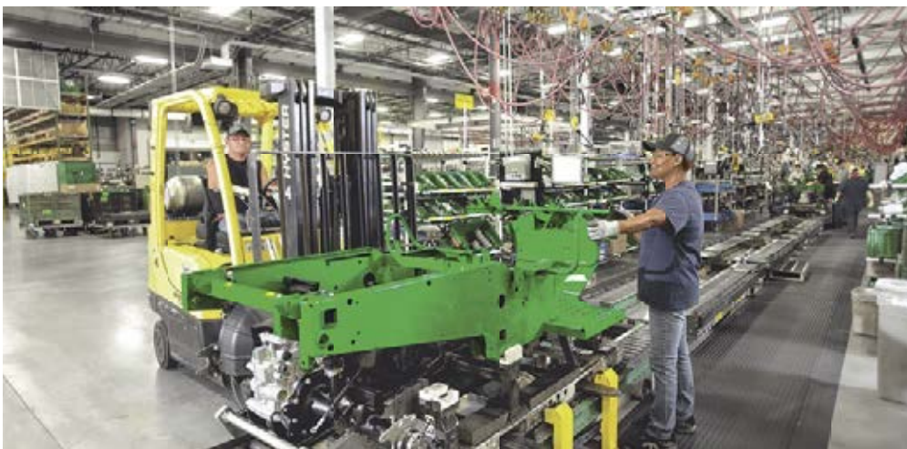
A traditional (T-) Series frame and drive train are placed on assembly line. They will leave the line as fully-assembled T-Series Gator.
